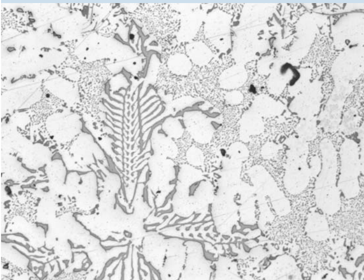
2 Dendritic cast iron (including 2 different eutectics in the residue melt area)
